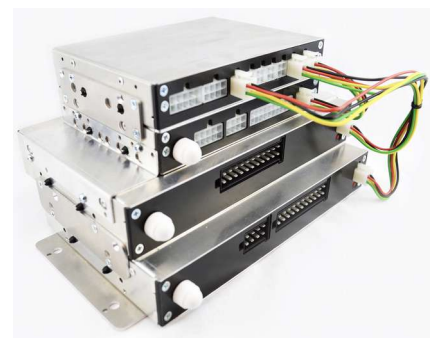
Several, partly different, EC2C I/O modules mounted as a tower.
